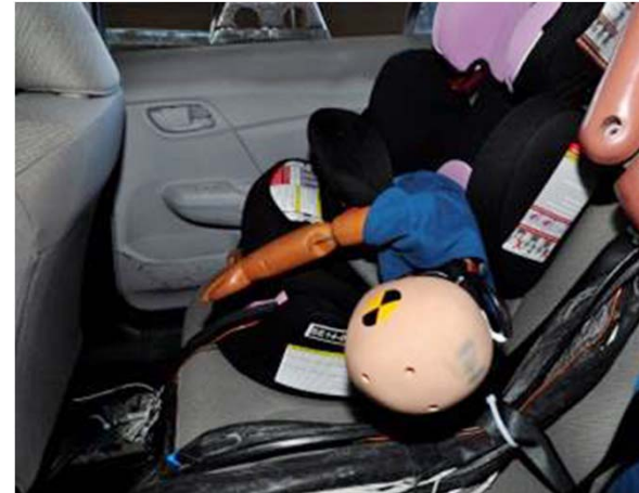
Partial ejection of the Q1,5 Dummy Left and US Crabi 18m Dummy Right
