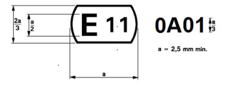
The above approval mark affixed to a gas-discharge light source indicates that the light source has been approved in the United Kingdom (E11) under the approval code 0A01. The first character of the approval code indicates that the approval was granted in accordance with the requirements of Regulation No 99 in its original form."
