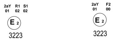
Marking of an interdependent lamp comprising part of an interdependent lamp system providing:
