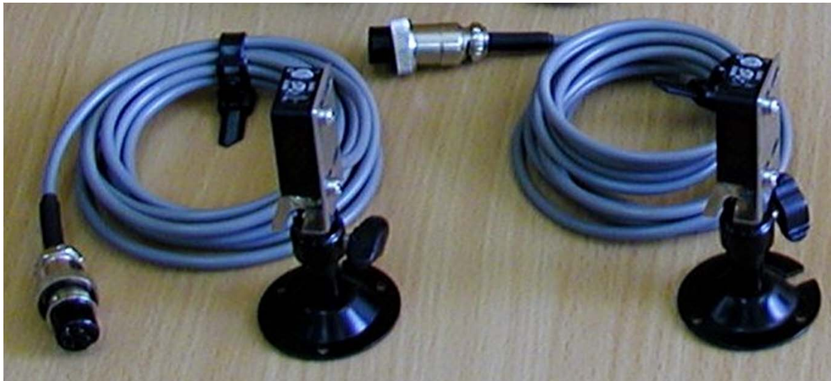
Sensors with magnetic supports for revolution measuring
