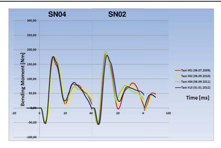
High repeatability during the primary impact phase SN04 curve characteristics comparable to SN02 during the impact phase
