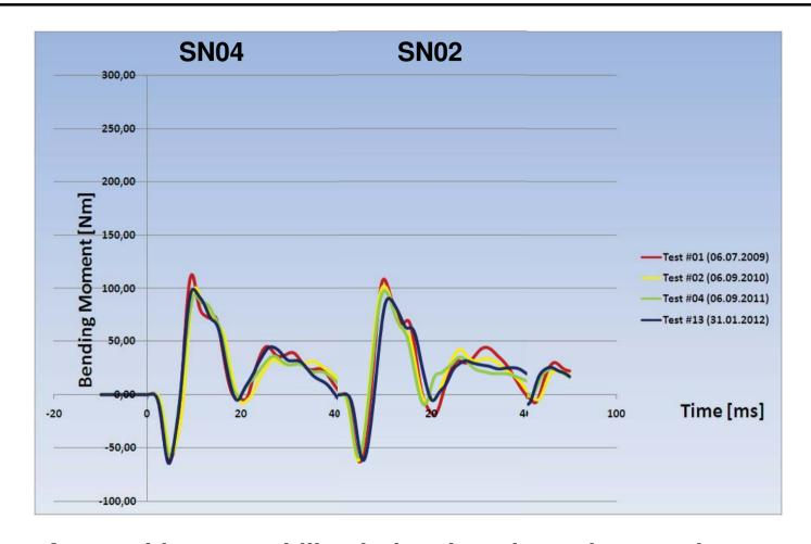
Acceptable repeatability during the primary impact phase Test #1 with maximum result
