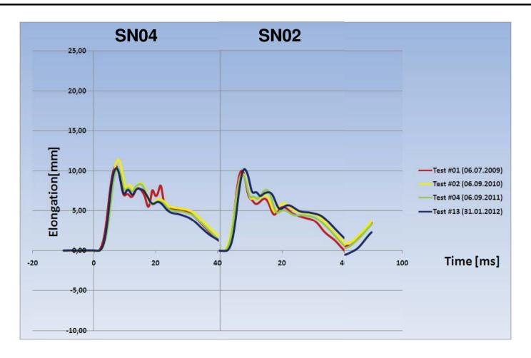
Acceptable repeatability during the impact phase Test #1 with different curve characteristics after the first peak SN04 curve characteristics comparable to SN02 during the impact phase
