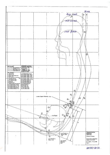
Based on this UMTRI-86-39 study, the position of the back-of-head of the large male, compared to the mid-sized male, is found here on a "distance x" which is 31mm more rearwards.
