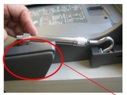
With the provision of Paragraph 8.2.9.2., measurement in operation as indicated in the user's manual may become difficult in some products. In this case, use of a hook of the geometry that enables such measurement should be allowed.
