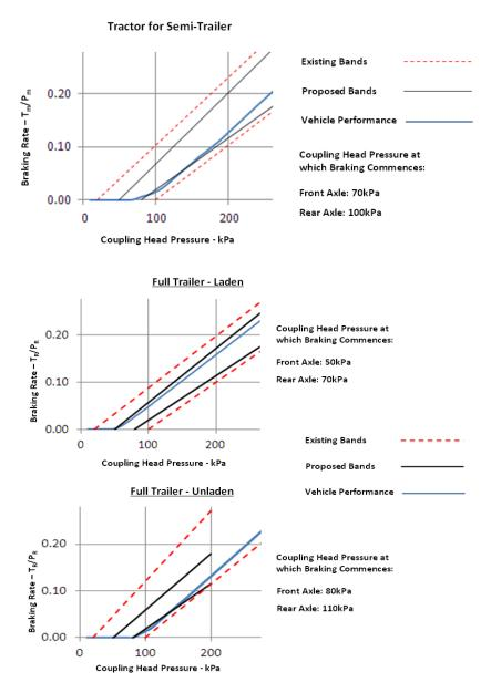
From the above it can be seen that it is often the case that following the initial generation of a braking force the vehicle performance is not linear, and is the result of the respective axles on the vehicle commencing braking at different coupling head pressures. These characteristics are typical of any conventional pneumatic braking system and could only be overcome by the use of electronic control.
