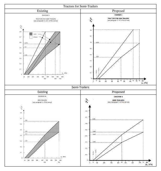
In the case of towing vehicles, trailers (including centre axle trailers) and tractors for semi-trailers it is proposed to remove the co-ordinates associated with the unladen bands and, by the amendment proposed for paragraph 1.1 of Annex 13, it would be required to fulfil the laden compatibility band up to a coupling head pressure of 200kPa for all states of load other than
