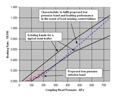
It can be seen that the relationship of coupling head pressure to generated braking rate is no longer the typical linear relationship. Such a characteristic can only be produced by the brake control system by modifying the
