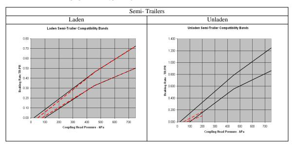
The broken red line represents the range of the bands proposed while the solid lines represent the bands determined using the methodology currently prescribed within Annex 10 to Regulation 13.
