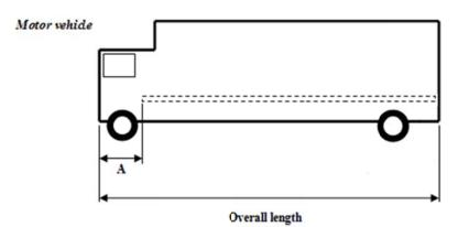
A is the distance between the foremost conspicuity marking and the front end of the vehicle. The maximum value of A is 2400 mm (see paragraph 6.21.4.2.1.1.)."
