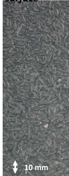
Porous elastic road surface
