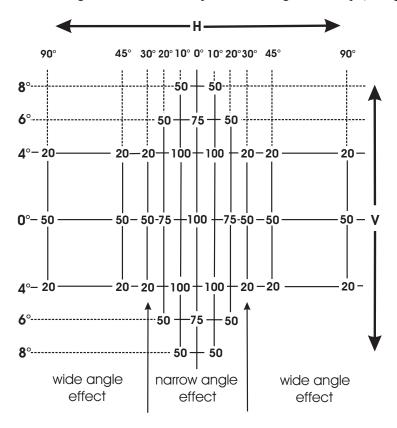
Minimum horizontal angular range of category "narrow angle effect" is  $30^{\circ}$  left to  $30^{\circ}$  right and for category "wide angle effect"  $90^{\circ}$  directed outwards the vehicle and  $30^{\circ}$  to the inside.
