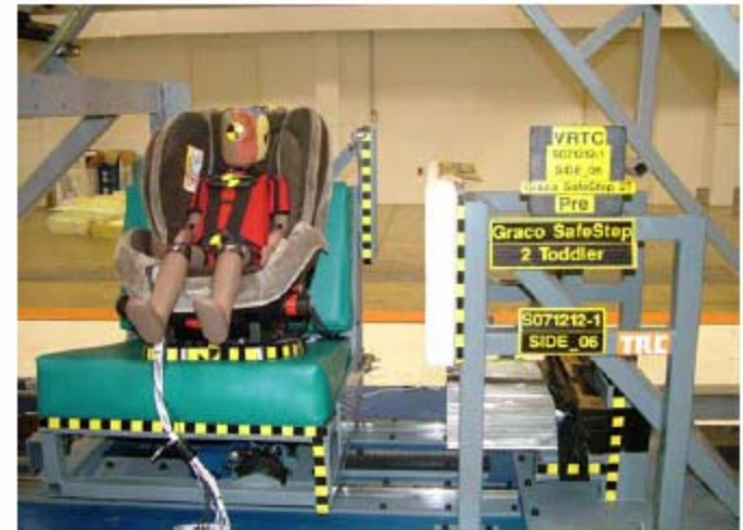
Figure 2. NHTSA's Side Impact Sled Buck Set-up.
