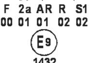
The above example corresponds to the marking of a lens intended to be used in different types of lamps. The approval marks indicate that the device was approved in Spain (E9) under approval number 1432 and comprises:
