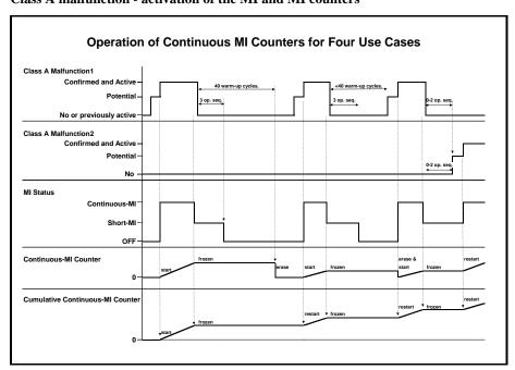
Note: Details related to the deactivation of the continuous MI are illustrated in Figure 4B below in the specific case where a potential state is present."
