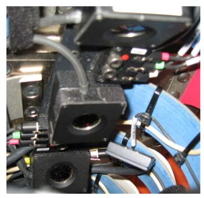
RibEye sensor array attached to spine box
