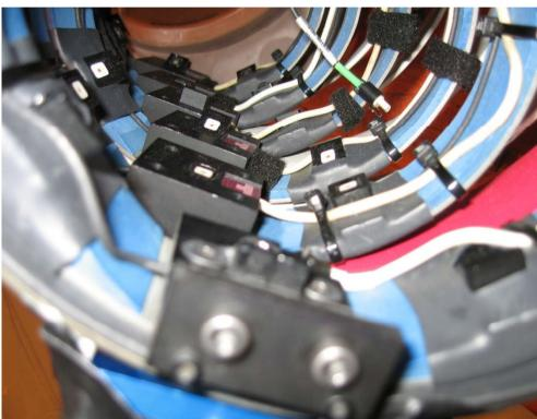
RibEye LEDs attached to inner rib
