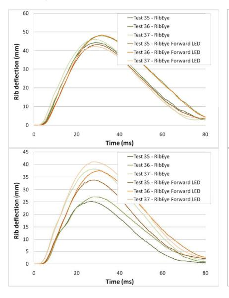
In the +30 and +20 degree conditions, with the dummy on the certification bench, the middle LED position gave approximately equal or greater resultant deflection measurements than the forward of lateral LED
