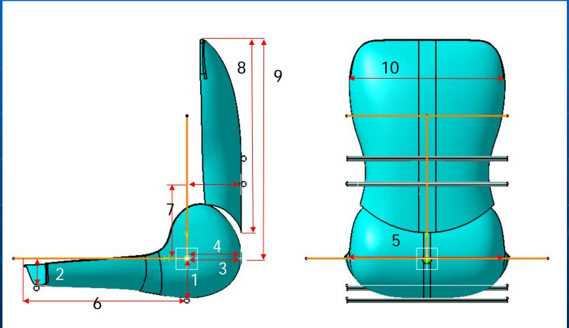
Used control points in fixture as control points for model + others
