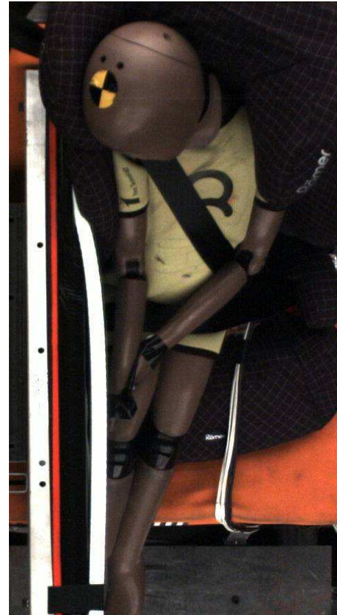
Q6 with additional bolster (100 mm) (dummy sitting height lifted artificially by 100 mm)
