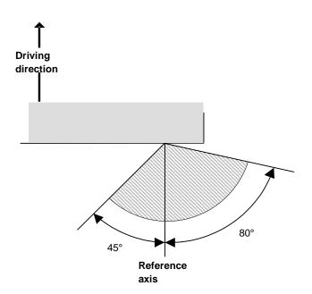
Under the H plane only for rear position lamps intended for  $M_1$  and  $N_1$  category of vehicles, and being installed at a mounting height less than 750mm above ground.
