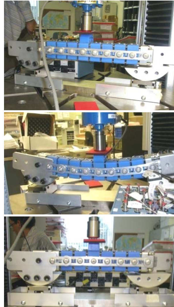
Tibia Assembly Quasi-static 3-point bending result in JARI corridors
