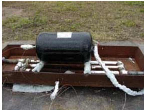
Figure 15: Hydrogen Tank Bonfire Test Apparatus
