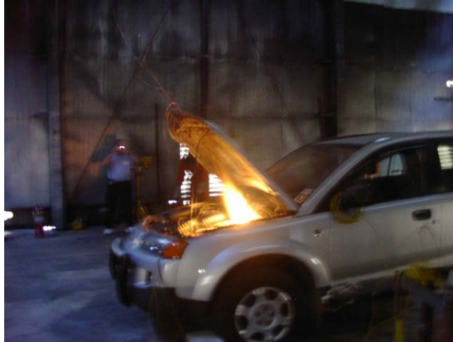
Figure 17: Fuel Line Leakage w Hood Open
