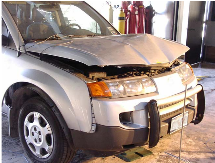
Figure 16: Damage done to Vehicle During H 2 Fire Test
