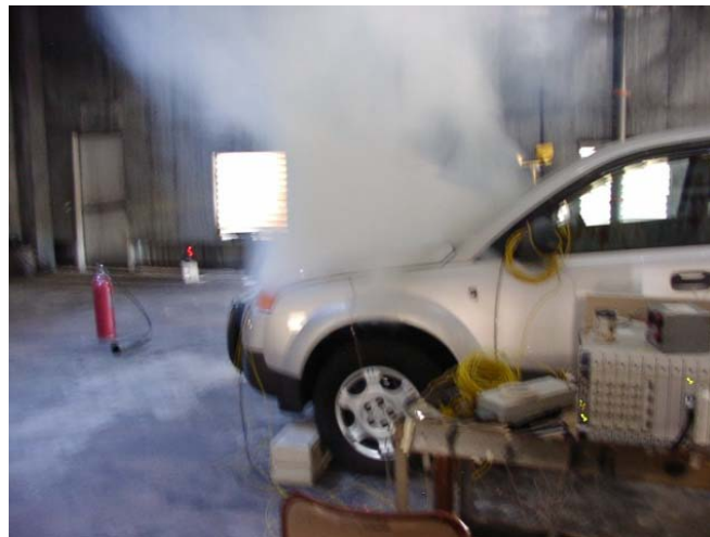
Figure 18: Fuel Line Leakage w Hood Closed
