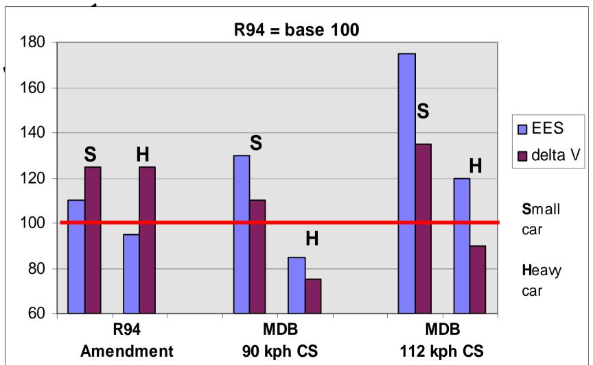
➤ Above the line 100, the test is severe than current R94
