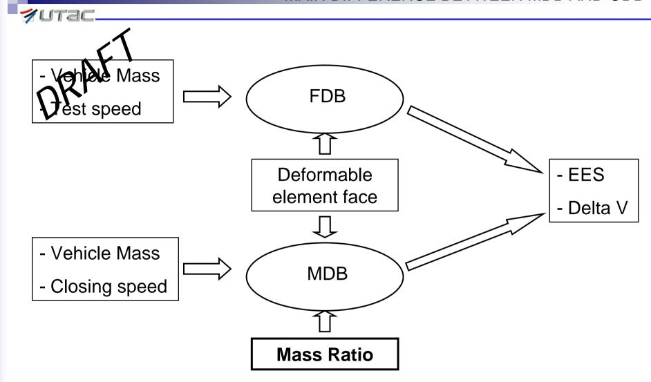
⇒Mass ratio parameter must be take into account to calculate test severity in addition of the energy absorbed by the barrier
