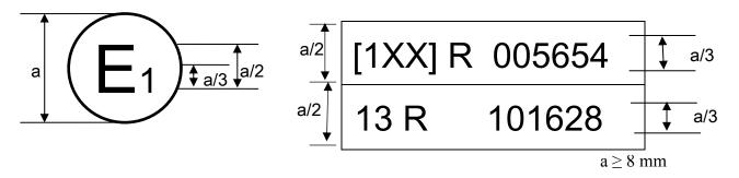
The above approval mark affixed to a vehicle shows that the vehicle type concerned has been approved in Germany (E1) pursuant to Regulations Nos. [1XX] and 13  $\underline{1}$ /. The approval numbers indicate that, at the dates when the respective approvals were given, Regulation No. [1XX] was in its original form and Regulation No. 13 included the 10 series of amendments.
