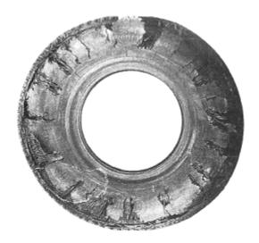
Photo 2: Ultimate tyre failure, resulting from driving on an under-inflated tyre.
