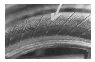
Photo 1: Fatigue cracks on a tyre inner liner, irreversible deterioration of the tyre not visible from outside, resulting from driving on an underinflated tyre.
