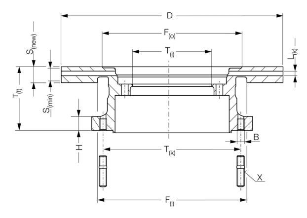
B Diameter of mounting bolt holes (or thread size in case of threaded holes)
