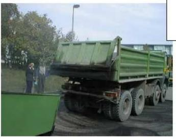
The rear part inclusive the rear under run protection device is completely in the mud!
