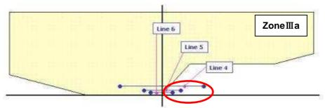
This means that there is an inconsistency between the existing dipped beam photometric requirement and adaptive driving beam photometric requirement.
