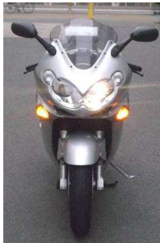
passing beam headlamp + amber position lamp
