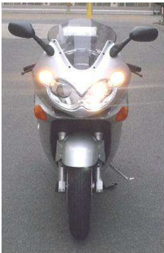
passing beam headlamp + white position lamp
