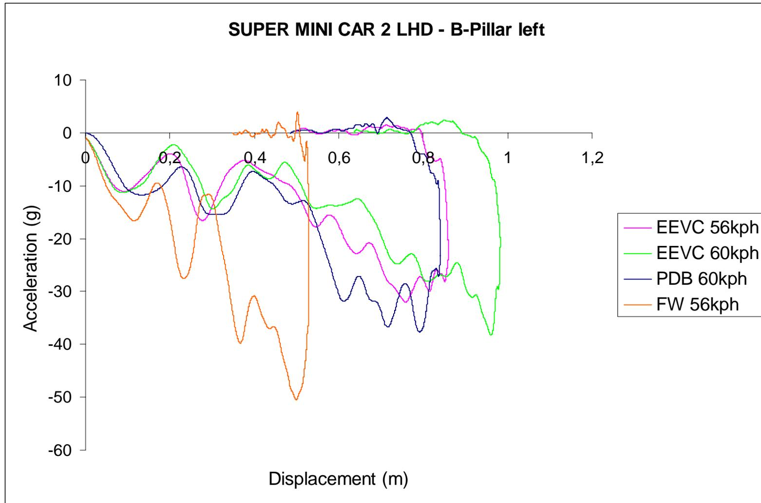
⇒ PDB test acceleration pulse is between ODB and FWRB
