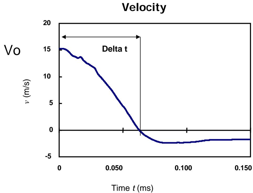
$$\text{Mean acceleration} = V_0 / \text{delta } t$$
