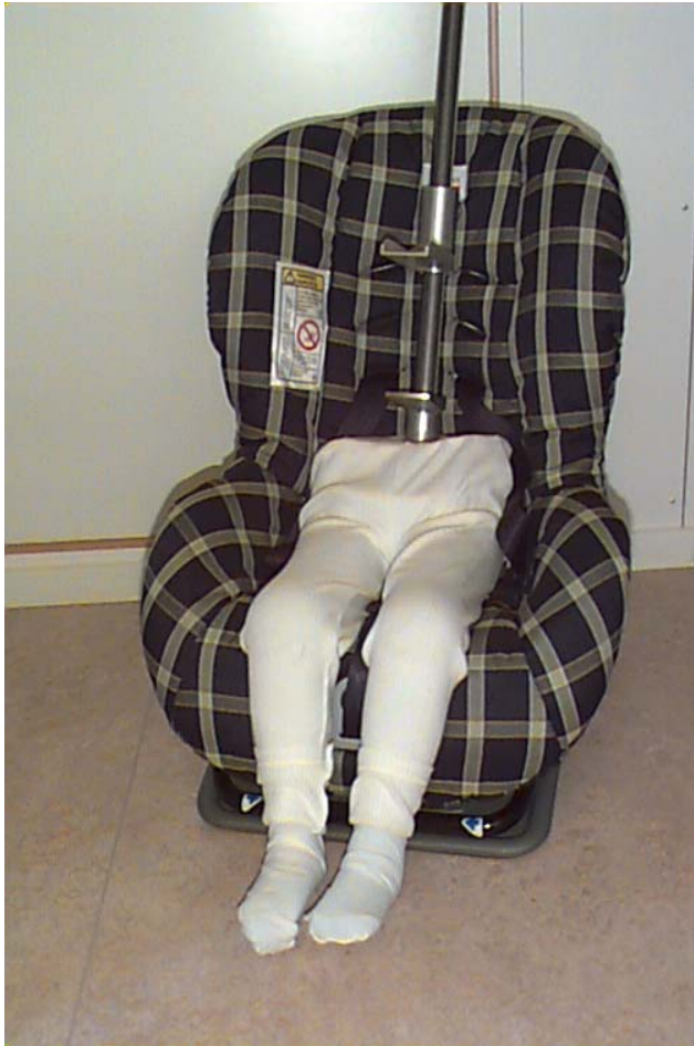
Figure 7 This VTI measuring device is used today to measure the seat back height. With minor modifications it can be used to measure the slot heights as well.
