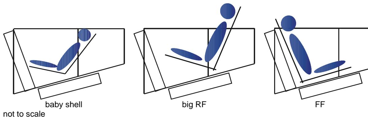
**Figure 7: Principle sketch showing CRS and dummy position depending on CRS type**
