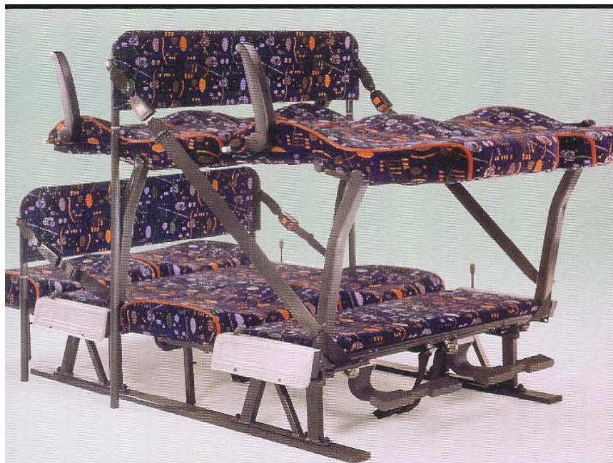
Example of safety partitions attached to the safety belt anchorages of the bus seats.
