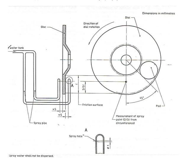
Notes on the installation of the disc brake water spray equipment:
