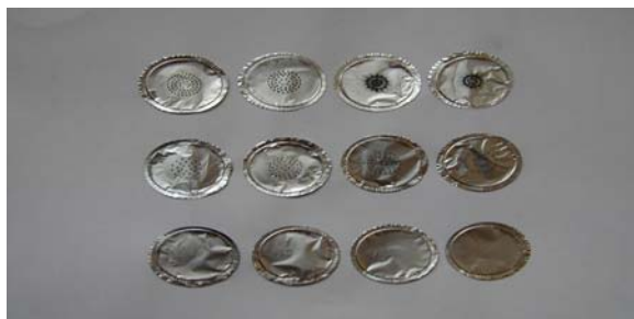
Fig. 3.4: PM particles with a diameter from 0.015 \mu\text{m} (collecting plate in the upper left-hand corner of the figure) to 6.4 \mu\text{m} (collecting plate in lower right-hand corner) are trapped in each stage of the ELPI impactor
