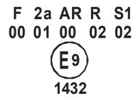
The above example corresponds to the marking of a lens intended to be used in different types of lamps. The approval marks indicate that the device was approved in Spain (E9) under approval number 1432 and comprises:
