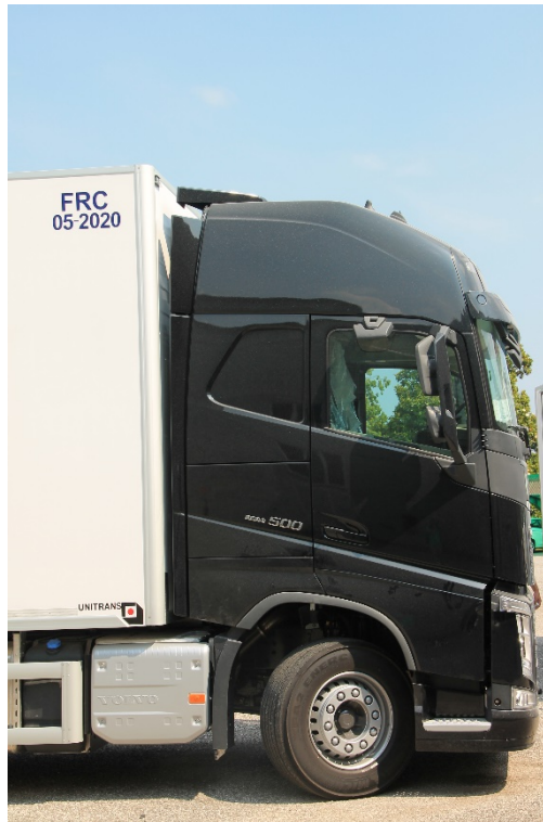
Class FRC (Class C mechanically refrigerated equipment with heavy insulation) certified equipment EuroMed RRU © EuroMed RRU
