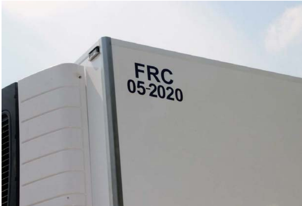
Class FRC (Class C mechanically refrigerated equipment with heavy insulation) certified equipment EuroMed RRU © EuroMed RRU
