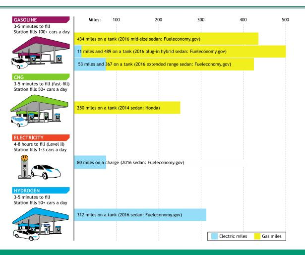
Range provided by a refill Gasoline and CNG provide the convenience of fast refill, while Battery Electric Vehicles require long periods of inactivity
