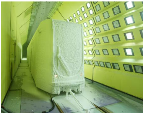
Climatic and air resistance tests at Rail Tec Arsenal in Vienna
