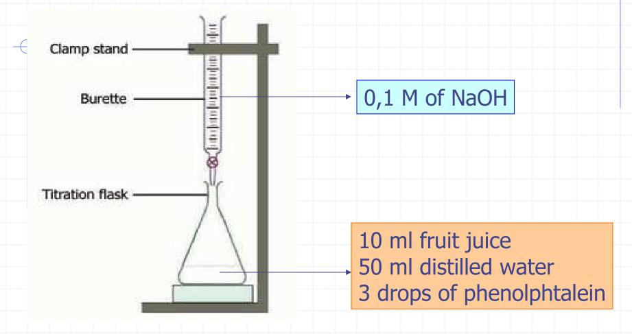
Drop NaOH (titre) into the titration flask until the colour changes (pH 8,1)
