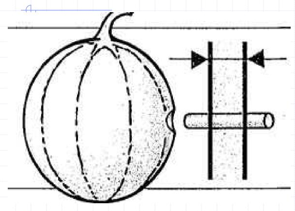
Using a small diameter metal borer (1 - 4 mm) a core of melon should be extracted from the equatorial axis area. Each end of the core should be discarded. The remaining flesh should be used to extract the juice for testing.
