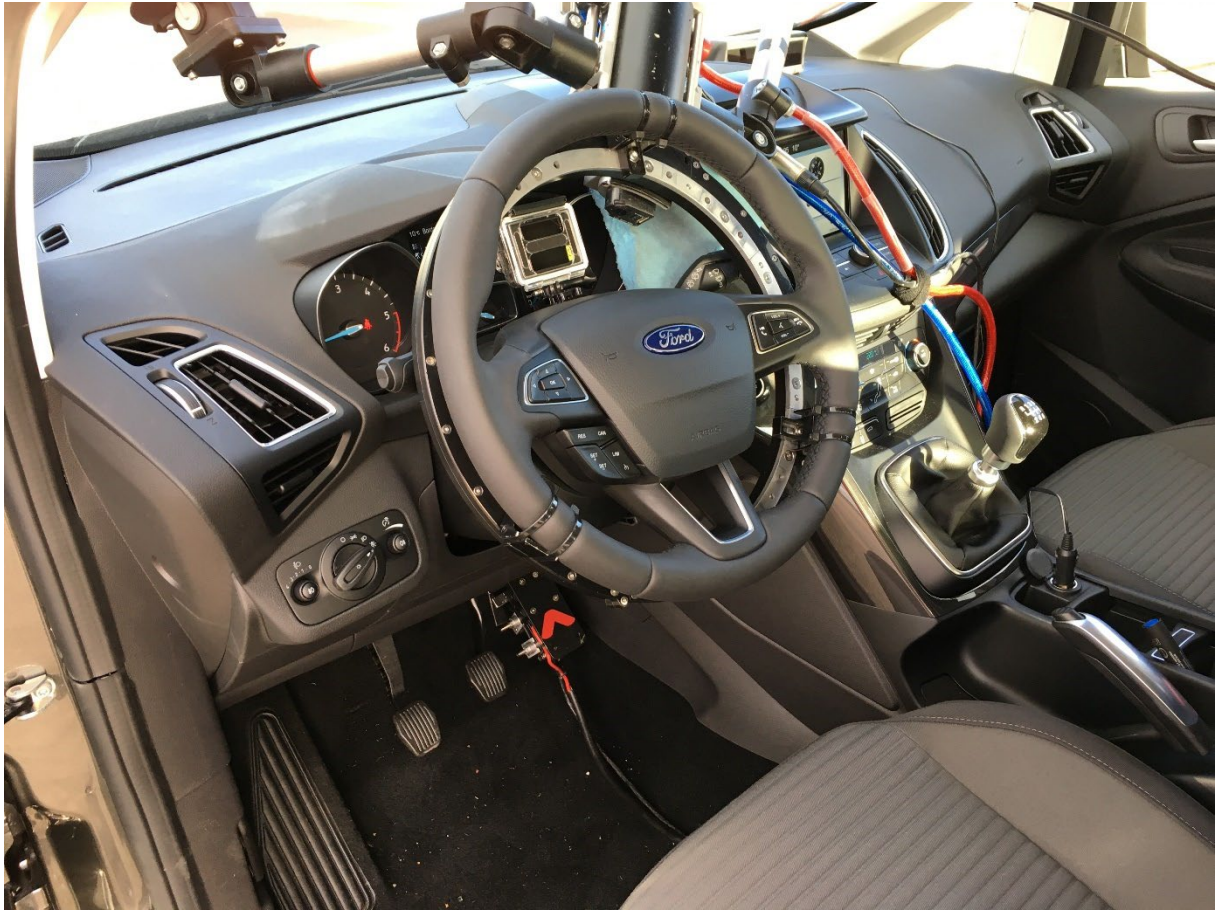
Figure 11: Vehico CS1200 steering robot, fitted in another vehicle
