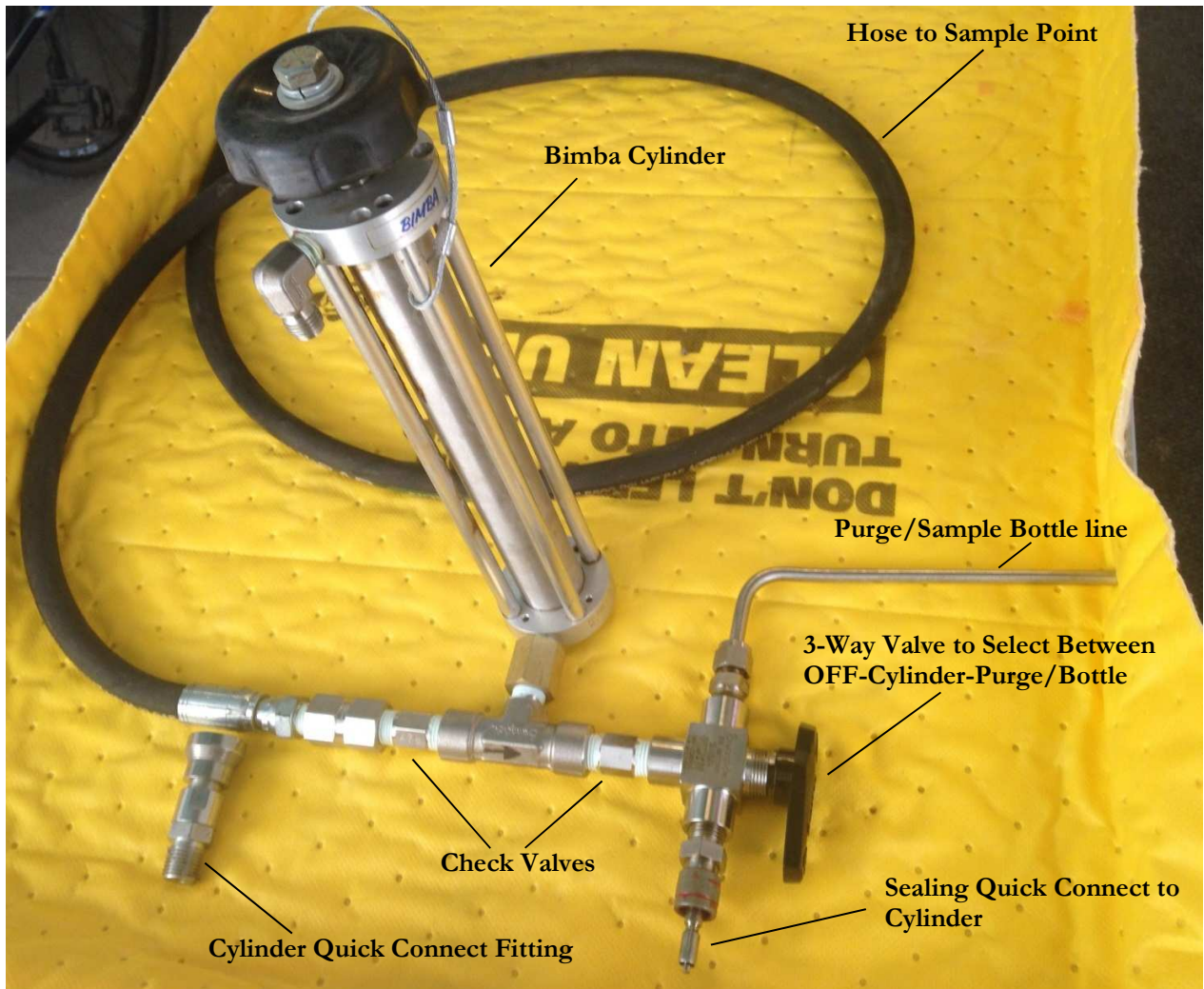
Figure 2: Sampling Assembly
