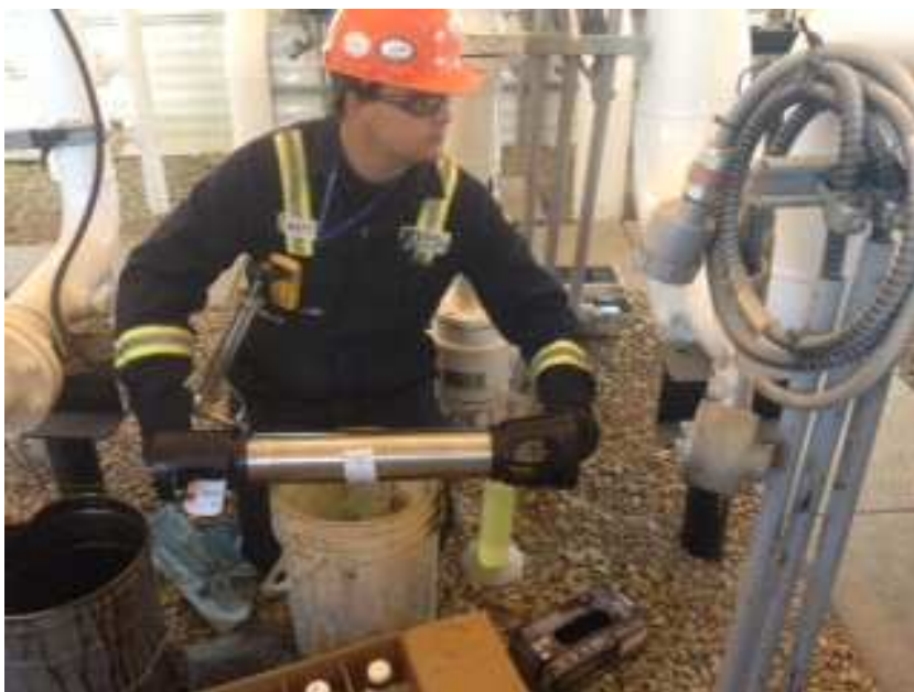
Figure 4: Pressurized Sample Collection at a Truck Terminal
