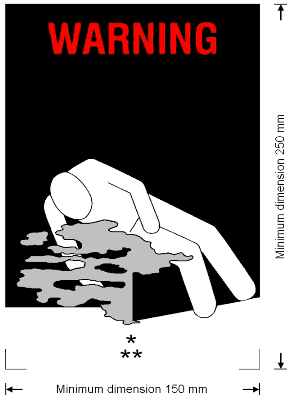
Coolant/conditioning warning mark for vehicles and containers
