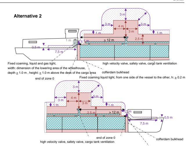
Fixed coaming liquid tight, from one side of the vessel to the other, h:  $\geq$  0,2 m
