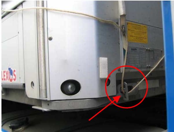
Lock tab secured by the TIR wire.
